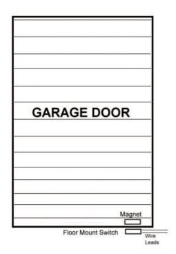
Mount contact on garage floor near the bottom of the garage door Mount magnet-bracket at bottom of garage door, above the contact Make sure gap between contact and magnet is not less than 1/4" Splice leads into alarm circuit.
